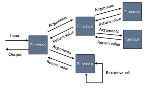
In functional programming individual tasks are small and achieved by passing data to a function which returns a result. This function typically does not change the state of the system or other functions.
